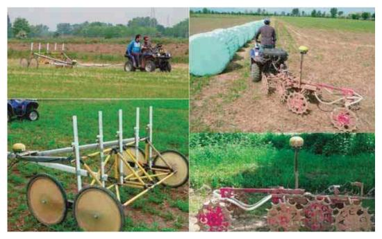
Figure 2. Geophysical instruments used during the survey. Left: the Automatic Magnetic Profiler (AMP© Geocarta), capable of recording up to 20ha each day. Right: the Automatic Resistivity Profiler (ARP© Geocarta), capable of recording up to 4ha each day. To increase productivity within the project two ARP instruments were often used simultaneously.
